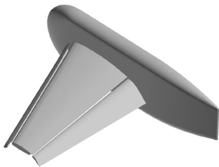
Fig. 1 NASA Trapezoidal Wing (Config.1)
