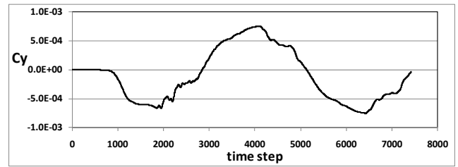
Fig.7 Time history of C_y in the cavitation tunnel (no FL, StdG, \theta = 0.0 deg., MSA)
