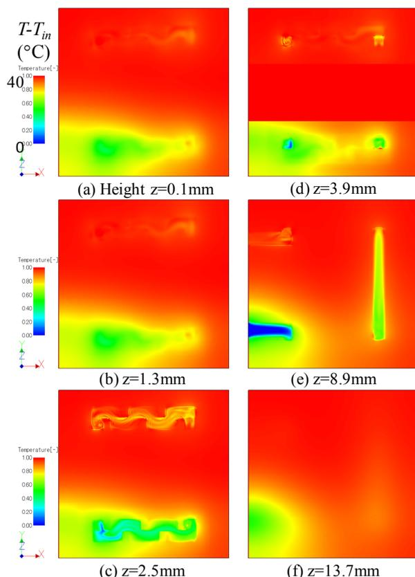
Fig. 11 The temperature distributions on horizontal cross section for  $Pr=2, Q_{in}=0.15$  l/min. and  $T_{in} = -10^\circ\text{C}$  at  $t = 0.848s$ .
