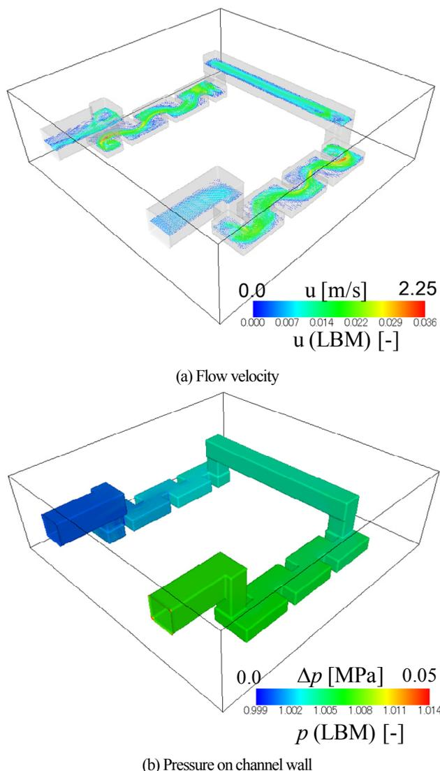
Fig. 5 The numerical results for  $Re=153.6$  ( $Q_{in}=0.3$ l/min).
