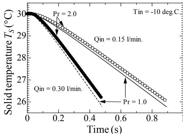
Fig. 6 The cooling rates dependent on  $Q_{in}$  and  $Pr$ , for  $T_{in}=-10^{\circ}C$  and I.C. Type (A).
