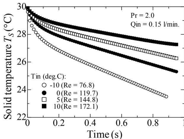
(a)  $Q_{in}=0.15$  l/min and  $T_{in}=-10^{\circ}\text{C}$  to  $+10^{\circ}\text{C}$ .
