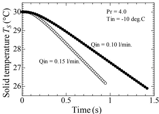
Fig. 8 The cooling rate dependent on  $Q_{in}$  for  $Pr=4.0$  and  $T_{in}=-10^{\circ}\text{C}$ .
