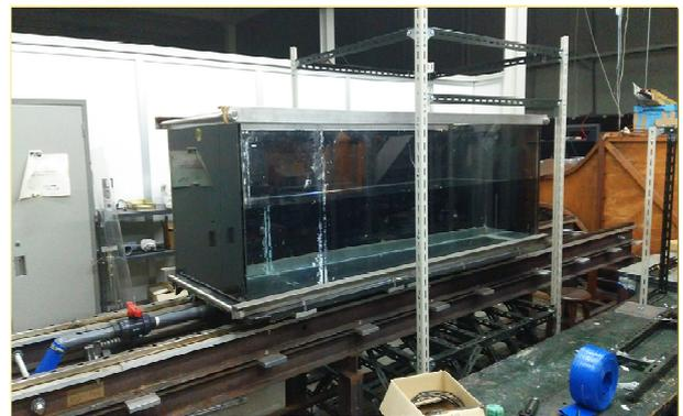
Fig. 7 Photograph of an experimental set-up with a moving water tank.
