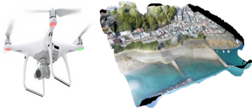
Fig. 6: Drone(left) and model using data by drone(right)
