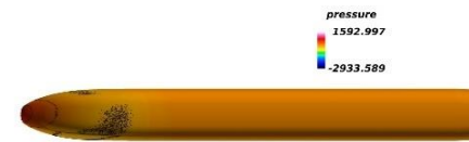
3) Surface Pressure contours (top view): vehicle has traversed half wavelength crosswind
