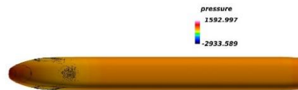
1) Surface Pressure contours (top view):, just before vehicle front approaches crosswind,
