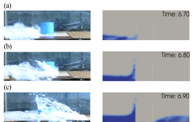
Fig. 3 Comparison of tsunami wave around the tank: (a) t = 6.7 s, (b) t = 6.8 s, (c) t = 6.9 s.
