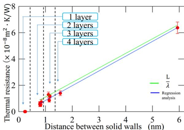
Fig. 5 Relationship between the thermal resistance of liquid and the distance between solid surfaces.
