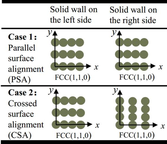
Fig. 2 Solid surfaces used in the simulation
