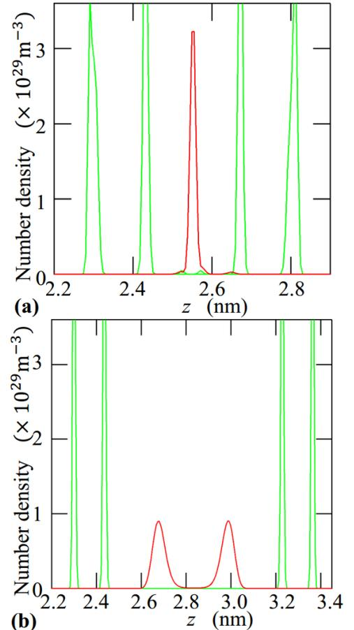
Fig. 3 The number density distribution of solid and liquid molecules (The green lines represent solid molecules, and the red lines represent liquid molecules).
