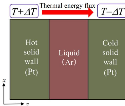
Fig. 1 Simulation system of heat transfer over liquid films between solid walls
