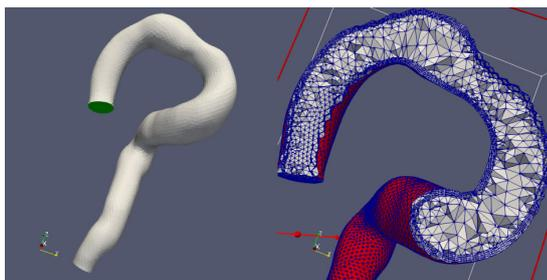
Fig. 1: Triangle surface and tetrahedral volume meshes
