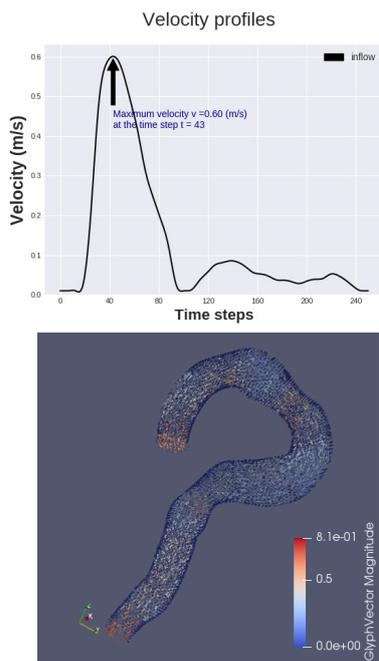
Fig. 2: Inlet velocity profile and the result flow pattern
