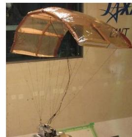
Fig. 1 Partially sealed parafoil.
