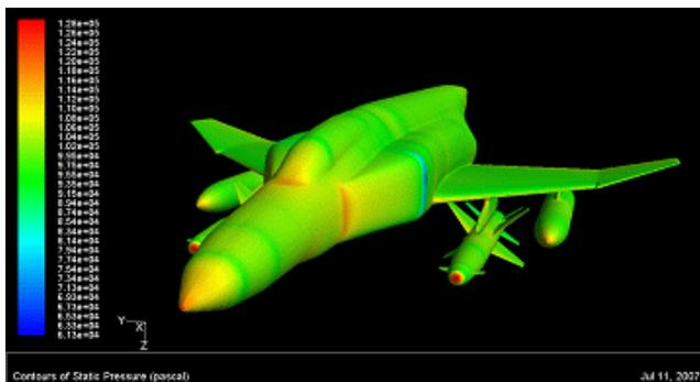
Fig. 6 The pressure contour of full configurations
