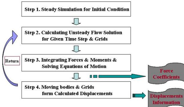
Fig. 3 Unsteady simulation procedure.
