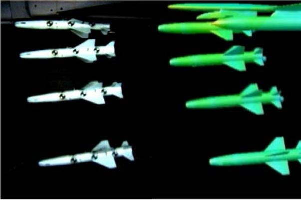
Fig.8 Comparison of experimental (left) and computational (right) separation results
