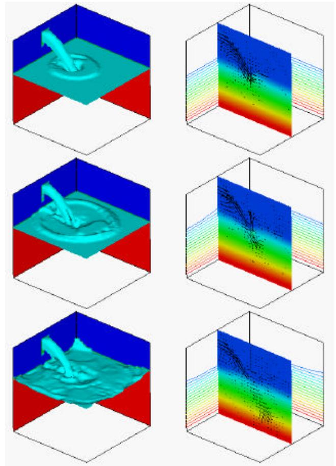
(a) Behavior of interface (b) Pressure and velocity vectors
