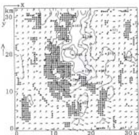
Fig.4-1 Area of strong ascending wind calculated by potential flow model
