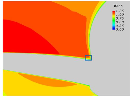
(a) Mach number distribution at mid-chord position of wing-root section (Small square is the size of view for (b) and (c)).
