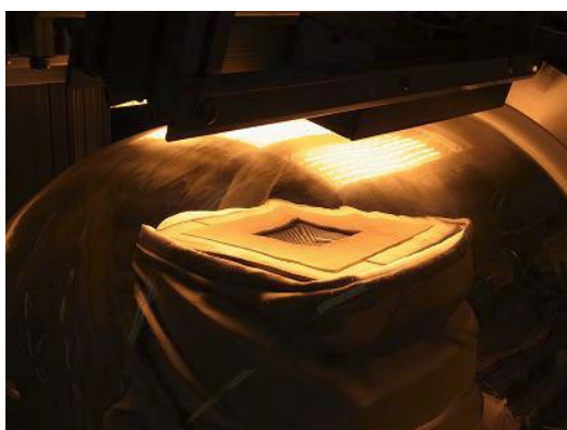
(b) Experimental Setup Fig. 6 Infrared lamp heating test (4) .
