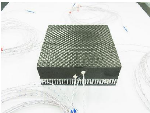
(a) NALT test piece for infrared lamp heating test.
