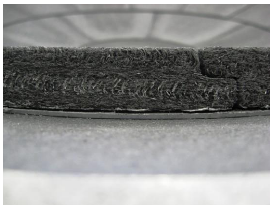
(a) Separation between C/C skin and insulator
