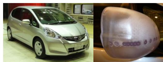
(a) FIT (b) Pressure hole
