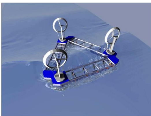
Fig.15 Simulation in severe wind and wave of a new semi-submerged floating body using RIAM-CMEN based on CIP method, by Prof. Hu at RIAM, Kyushu University
