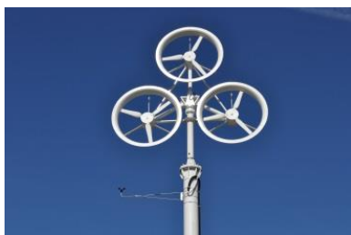
Fig. 9 3kW clustered Wind-Lens turbine using three 1kW wind lens turbines at Kyushu University.
