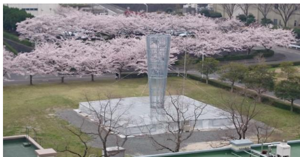
Fig.28 Field experiment using a prototype WST with 11m high tower and 15m square collector.
