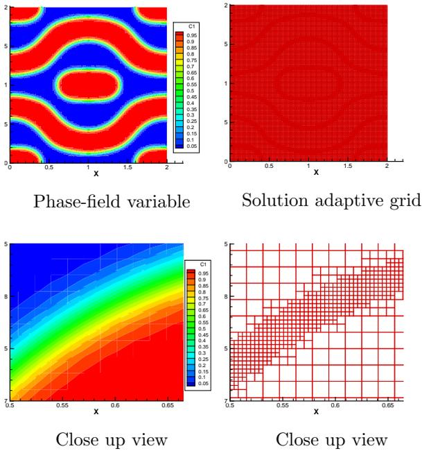
Fig. 2: Solution adaptive grid for  $t=0.5$
