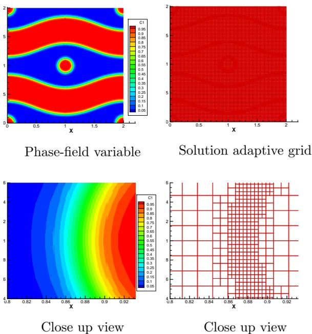
Fig. 3: Solution adaptive grid for  $t=5.0$
