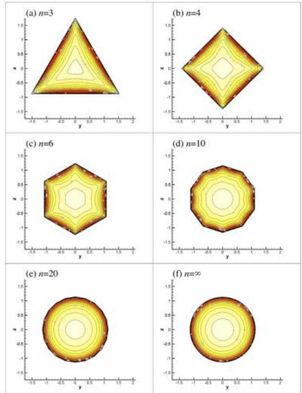
Fig. 6: Reynolds normal stress  $\overline{u'u'}$ .
