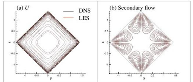
Fig. 2: Contour of the mean streamwise velocity and streamlines of the secondary flow.
