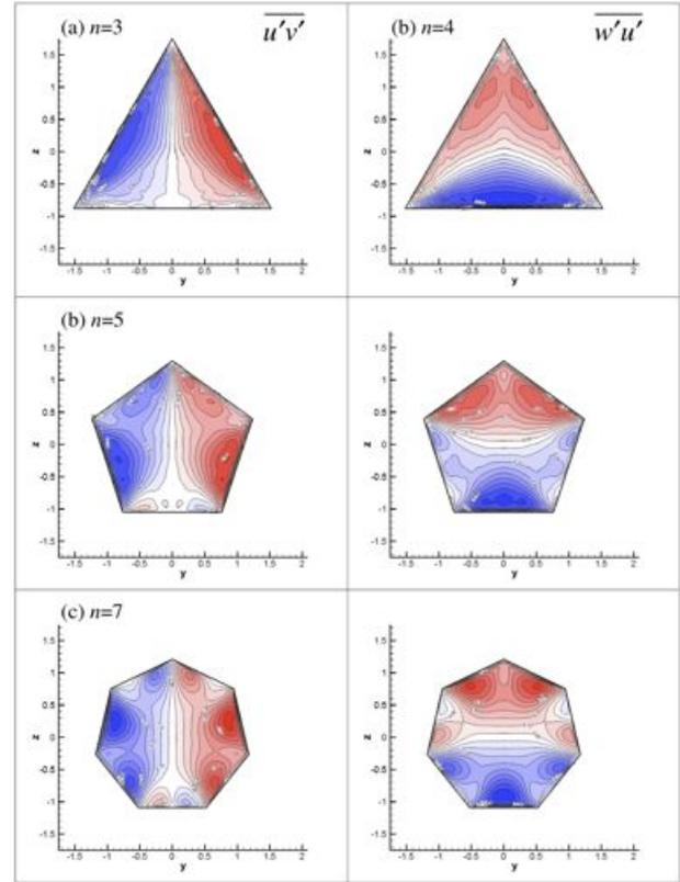
Fig. 10: Reynolds shear stresses  $\overline{u'v'}$  and  $\overline{w'u'}$ .
