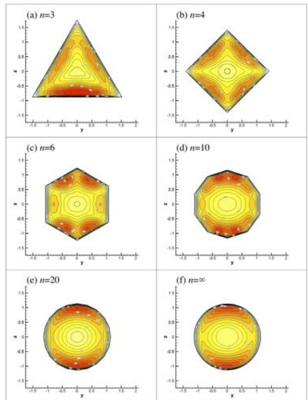
Fig. 7: Reynolds normal stress  $\overline{v'v'}$ .
