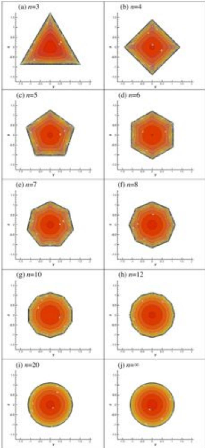
Fig. 5: Streamwise mean velocity  $U$  and secondary flow.
