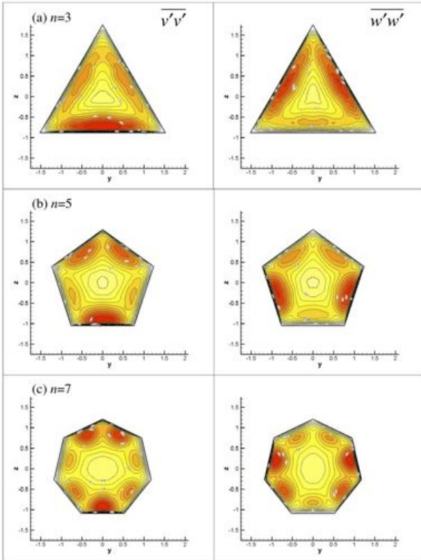
Fig. 8: Reynolds normal stresses  $\overline{v'v'}$  and  $\overline{w'w'}$ .
