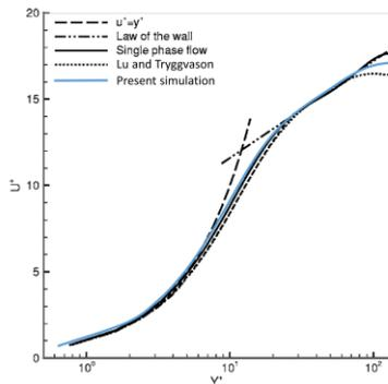
Fig. 3 Streamwise mean velocity distribution for void fraction of 1.5%. (black) Lu and Tryggvason, (blue) present simulation.
