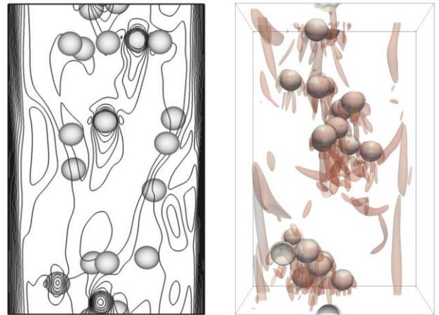
Fig. 1 The bubble distribution for void fraction of 1.5%. (left) Lu and Tryggvason (right) present simulation.
