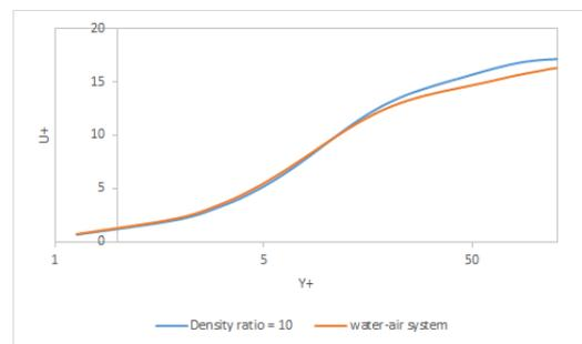
Fig. 6 Comparison of streamwise mean velocity distribution. (blue) density ratio of 10, (orange) water-air system.
