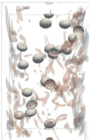
Fig. 4 The bubble distribution for water-air system with void fraction of 1.5%
