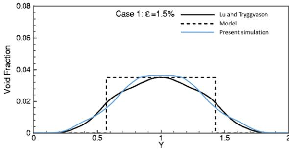
Fig. 2 Void fraction distribution for void fraction of 1.5%. (black) Lu and Tryggvason, (blue) present simulation.
