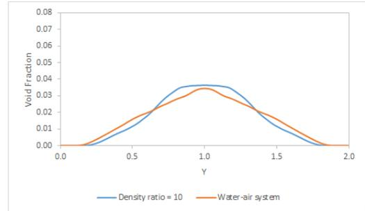
Fig. 5 Comparison of void fraction distribution. (blue) density ratio of 10, (orange) water-air system.
