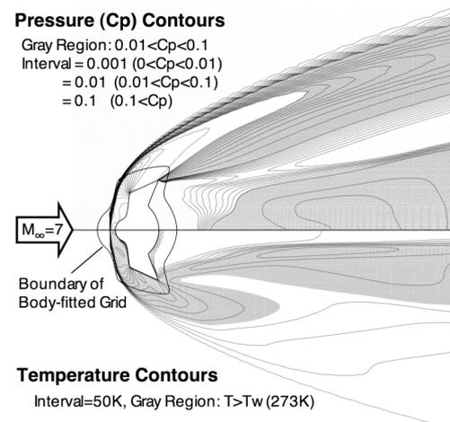
Fig. 2 Pressure and Temperature Contours
