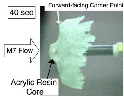
Fig. 1 Shape of ice piece (40 sec after injection into flow)
