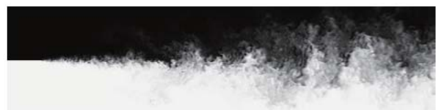
Fig. 2 Instantaneous scalar field for the mixing layer downstream of the fractal square grid
