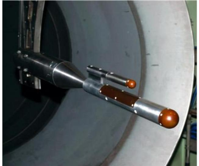
Fig. 5: Two hemisphere-cylinder model
