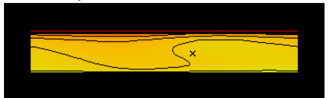
Fig. 6 Temperature distribution over the free surface during one cycle ( \tau_0 =one period)
