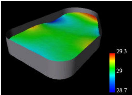
Fig.8 Computed configuration of free surface
