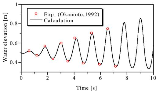
Fig.2 Time history of the water elevation at the left hand-side wall
