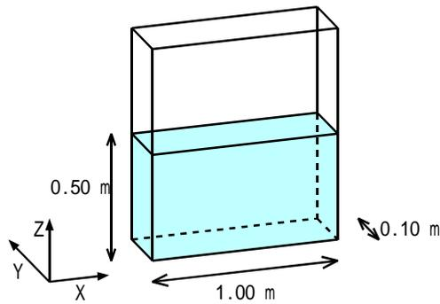
Fig.1 Numerical model of rectangular tank
