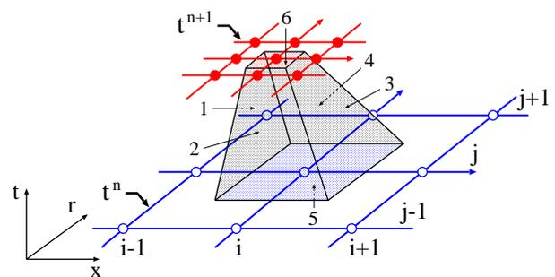
Fig. 1: Control volume in space-time system
