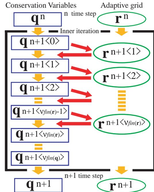
Fig. 2: Inner iteration process
