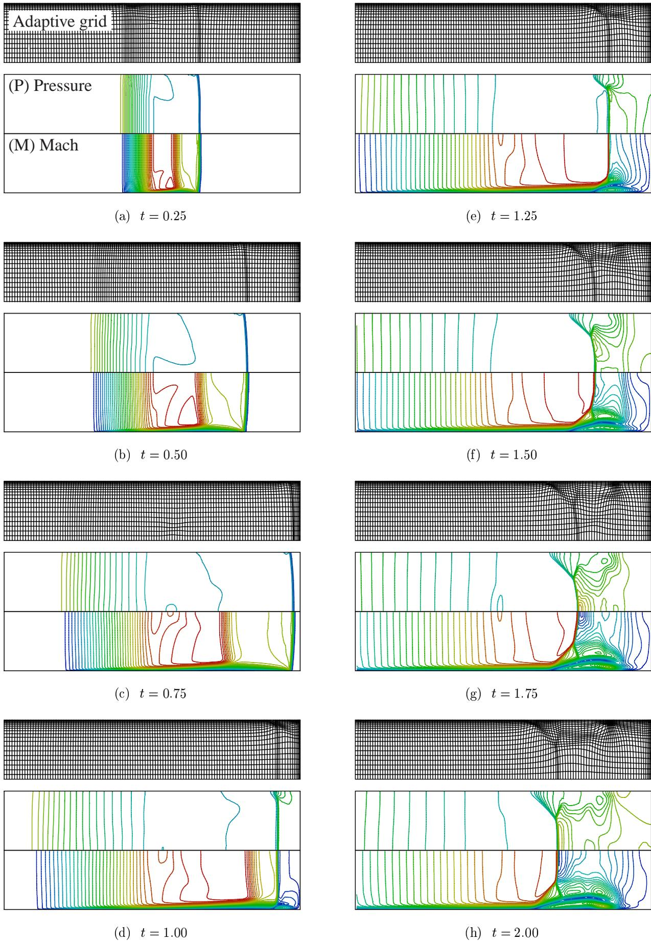
Fig. 6: Movement of solutions and solution-adapted mesh
