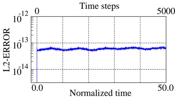
Fig. 3: History of L2-ERROR of density from initial condition
