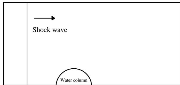
Fig. 6 Schematic diagram of initial conditions of the numerical simulation.
