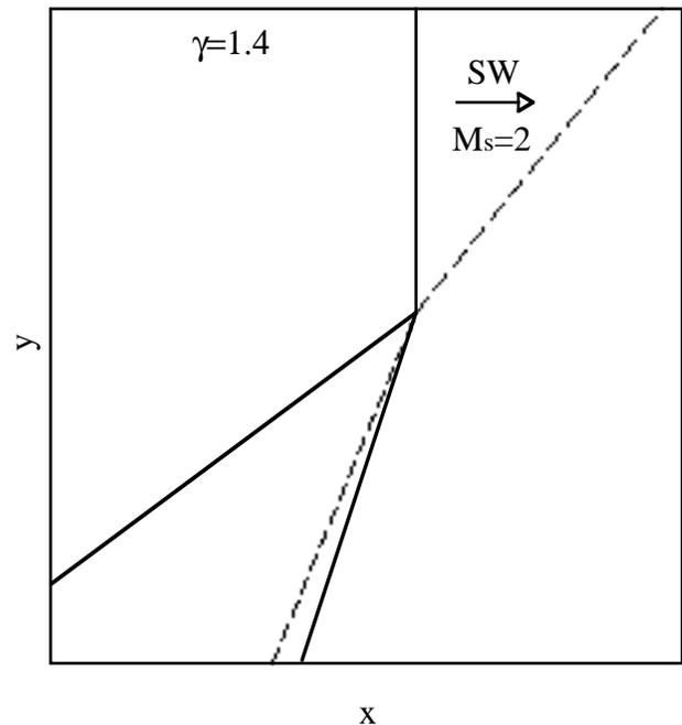
Fig. 3 Final condition of shock wave interaction with a gaseous wedge.
