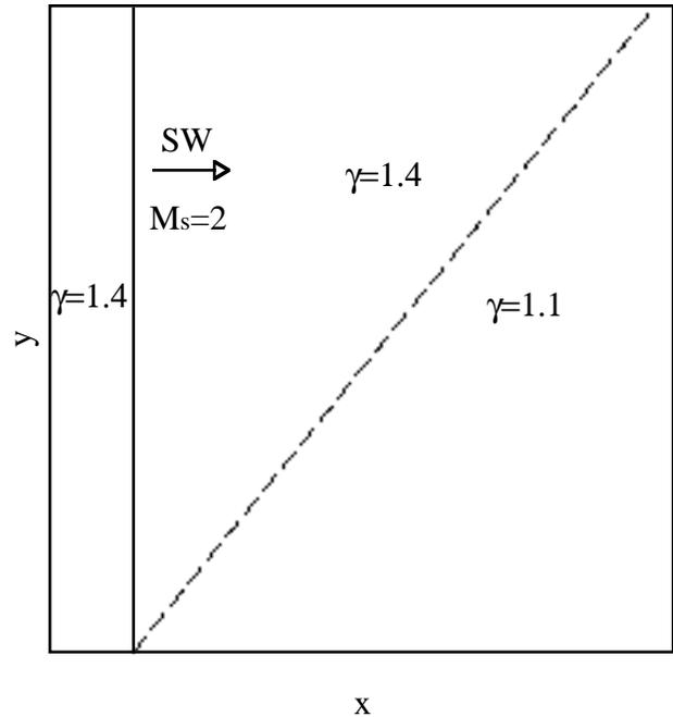
Fig. 2 Initial conditions for shock wave interaction with a gaseous wedge.
