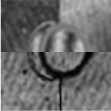
Fig. 9 Experimental results at  $t=4 \mu\text{s}$ : interferogram (top); unreconstructed hologram (bottom)
