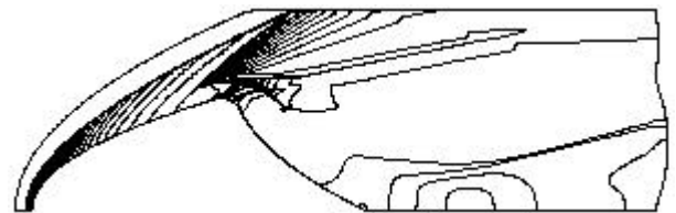
Fig.3 Pressure contours in the steady state flow field. (max. = 180818 Pa, min. = 408 Pa, incre. = 3608 Pa)
