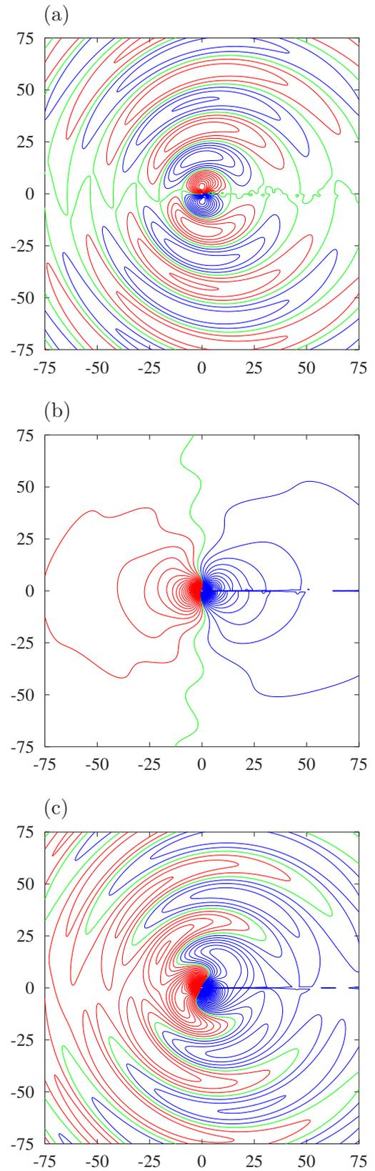
Fig. 2: Isobars with respect to the ambient pressure level, computed from the Ffowcs Williams–Hawkins dipole equation: (a) propagating term  $\Delta p_1$ ; (b) pseudo sound term  $\Delta p_2 + \Delta p_3$ ; (c) total dipole  $\Delta p_{FWH}$ . Contours at intervals of  $5 \times 10^{-5}$ : —, positive; —, negative; —, 0
