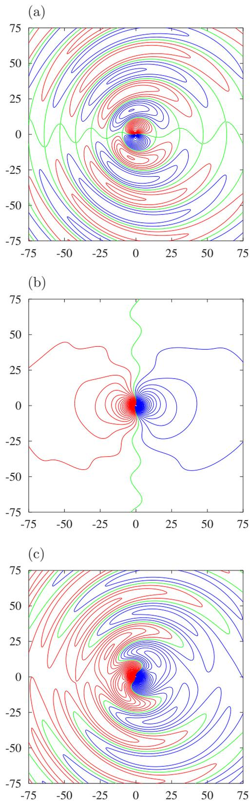
Fig. 4: Isobars with respect to the ambient pressure level, computed from the modified Curle's dipole: (a) propagation term  $\Delta p_{C1}$ ; (b) pseudo sound term  $\Delta p_{C2} + \Delta p_{C3}$ ; (c) total dipole  $\Delta p_{Curle}$ . Contours at intervals of  $5 \times 10^{-5}$ : —, positive; —, negative; —, 0
