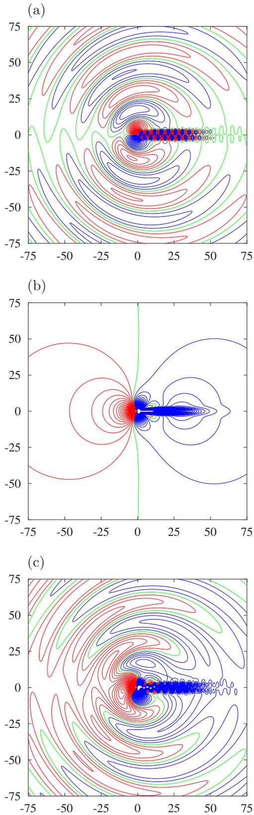
Fig. 1: Isobars with respect to the ambient pressure level  $p_0$ , obtained by DNS: (a) fluctuating pressure  $\Delta p' = \Delta p - \overline{\Delta p}$ ; (b) mean pressure  $\overline{\Delta p}$ ; (c) total pressure  $\Delta p = p - p_0$ .  $M = 0.2$ ,  $Re = 150$ ,  $t = 2000$ . Contours at intervals of  $5 \times 10^{-5}$ : —, positive; —, negative; —, 0
