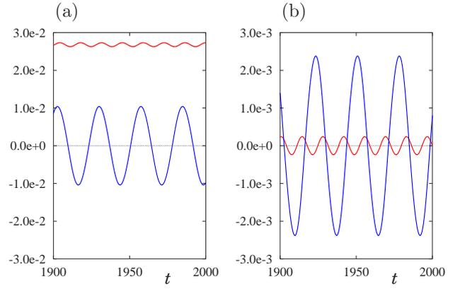
Fig. 3: Time histories of (a) forces on cylinder and (b) their time-derivatives: —, lift; —, drag.  $M = 0.2$ ,  $Re = 150$ .
