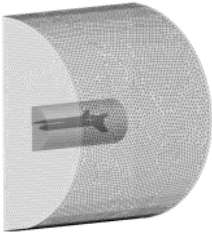
Fig. 9 Overset grids for the supersonic airplane (outer cylindrical region) and rocket booster (inner cylindrical region)
