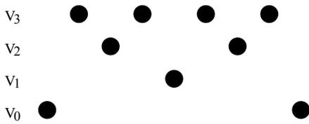
Fig.3 One-to-one relation between wavelet coefficients and grid points up to third level
