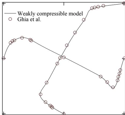
Fig.18 Mean velocity profile at center of cavity
