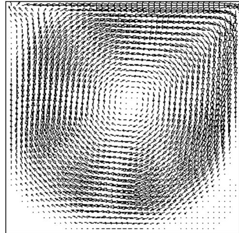
Fig.16 Velocity vector with  $Re = 1000, M = 0.1$
