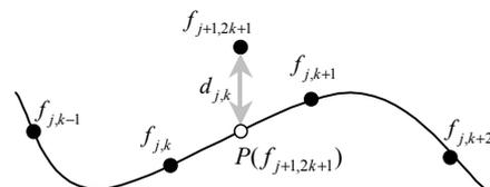
Fig.2 Wavelet coefficient by interpolating wavelets
