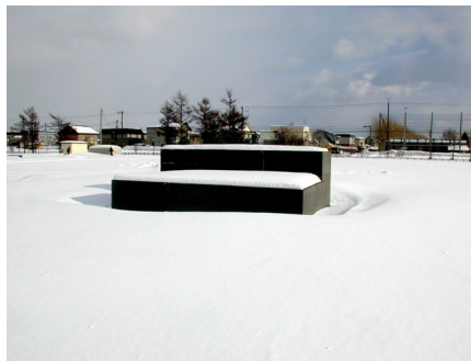
Photo 2 Field observation model for snowdrift.
