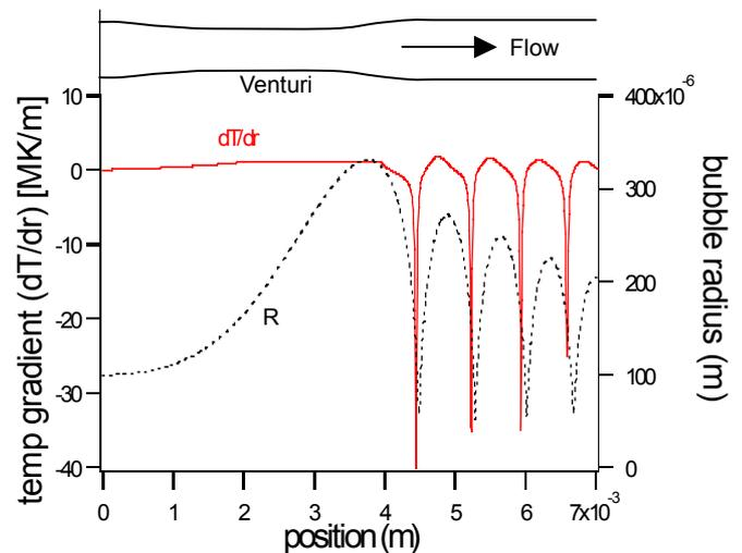
Fig. 5 Profile of temperature gradient at bubble wall and bubble radius in venturi tube computed by the present model.
