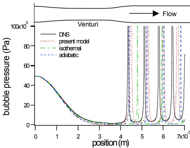
Fig. 3 Comparison of gas pressure inside bubble distributions in tested venturi amount different simulation methods.
