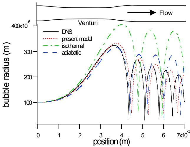
Fig. 2 Comparison of bubble radius distributions in tested venturi amount different simulation methods.
