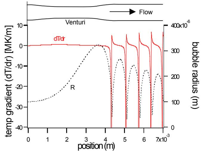
Fig. 4 Profile of temperature gradient at bubble wall and bubble radius in venturi tube computed by DNS.
