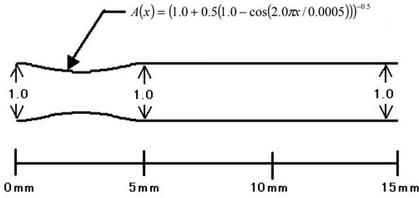
Fig. 1 Schematic of venturi tube
