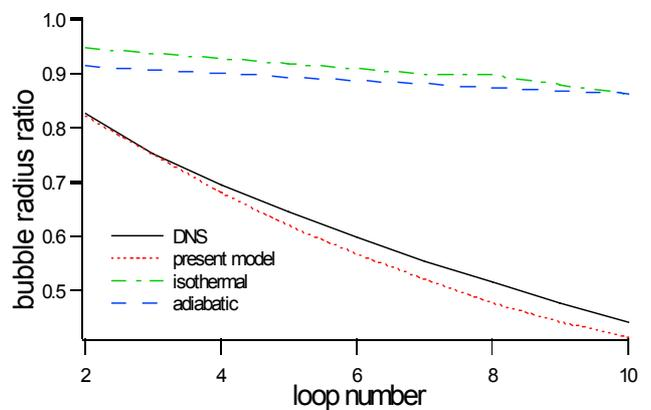
Fig. 7 Maximum bubble radius ( $R_{max(i)}$ ) of each oscillation loop relative to the maximum bubble radius ( $R_{max1}$ ) the first loop.
