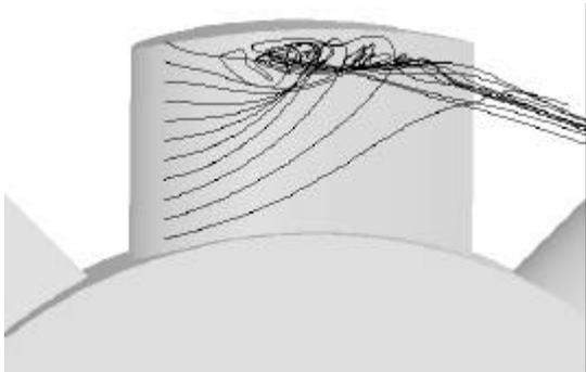
Fig. 4 Vortex flow created on the blade going downstream
