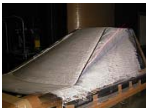
Fig. 12: Flow pattern: (a) oilflow in experiment; (b) streamline near wall in calculation (MTS, Case2)
